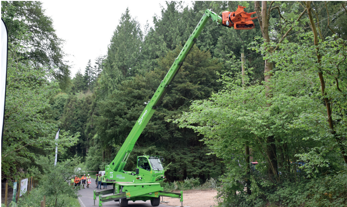
Left Woodcracker® CS580 Smart on the Merlo telehandler removing a limb above the telephone wire.
